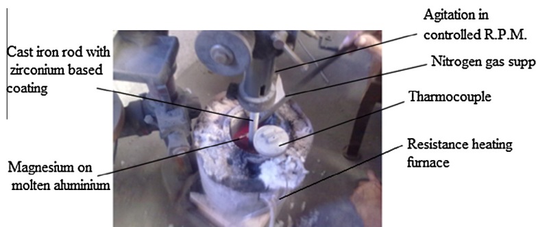
Fig. 1a. Photograph of set up for mixing of the SiC and Gr particle in aluminum.
