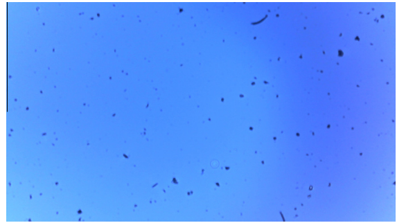
Fig. 1. A dust shadows image captured by using the sensing apparatus based on the HD CMOS optical sensor.
