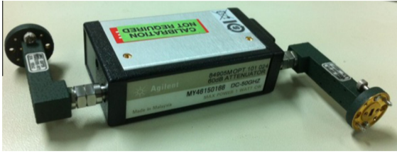
Fig. 1. Traveling standard for attenuation in WR-15 waveguide band.
