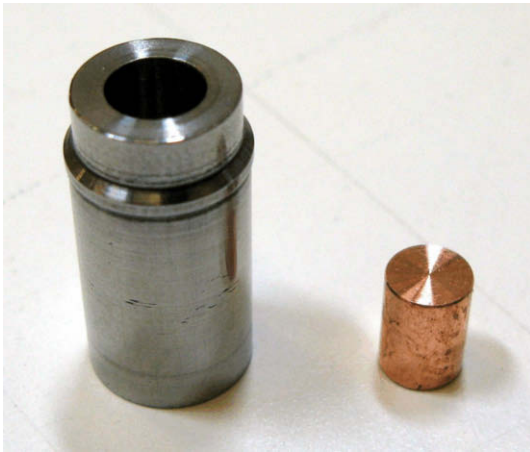
Fig. 1. Measurement cartridge and copper crusher cylinder.
