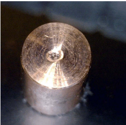
Fig. 2. Indent made by Glock-pistol firing pin on a copper cylinder head.
