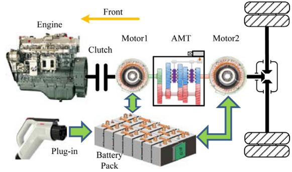
Fig. 1. The prototype of the single-shaft series-parallel powertrain.
