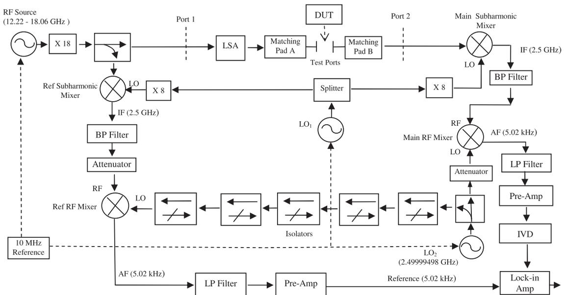
Fig. 1. Block diagram of a dual-channel millimeter-wave phase-shift measurement system from 220 GHz to 325 GHz.
