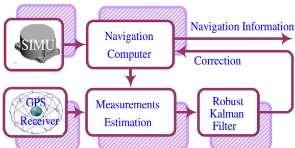
Fig. 1. SINS/GPS loose integration for in-motion alignment.
