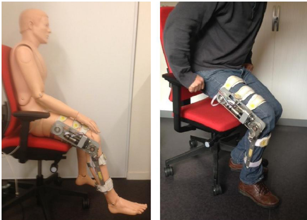
Fig. 1. The dummy and human wearing an actuated knee joint orthosis (EICoSI).
