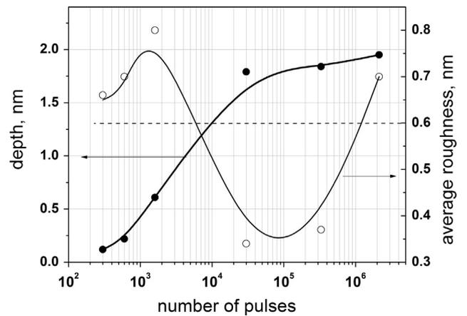
Fig. 3. Dependencies of mean crater depth (the thick line) and bottom roughness (the thin line) on pulse number,  $E=0.04 \text{ J/cm}^2$ .
