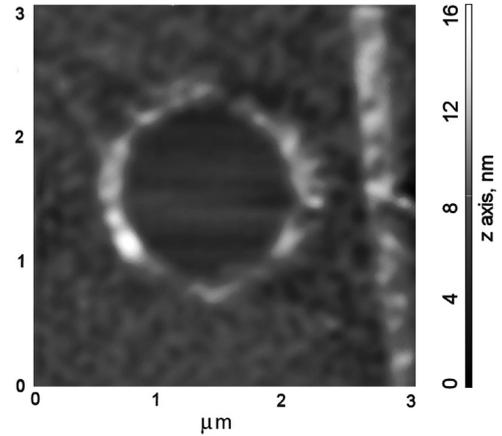
Fig. 2. AFM image of laser irradiated area at  $E=0.04 \text{ J/cm}^2$ , high exposition time ( $N=3 \times 10^5$ ).
