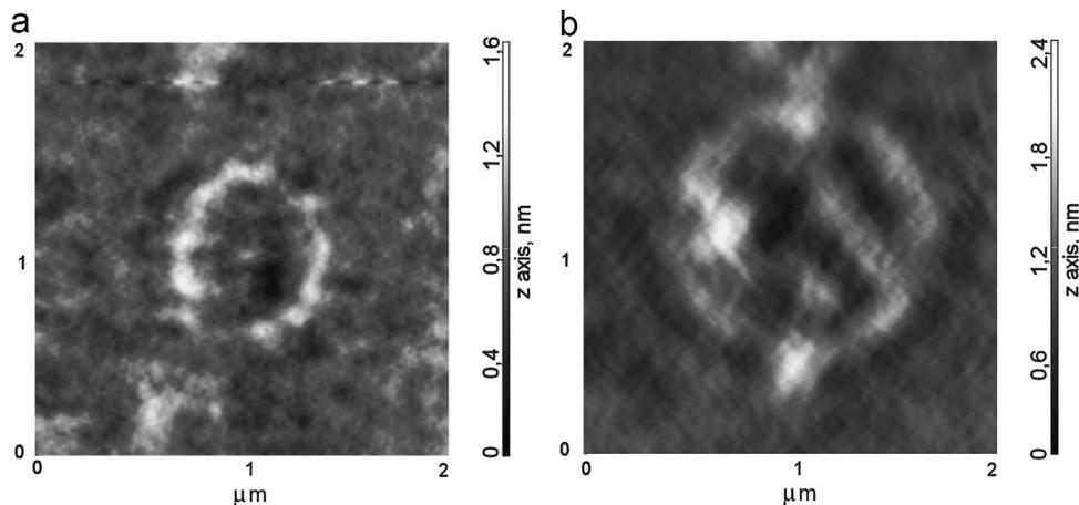
Fig. 1. AFM images of laser irradiated areas at  $E=0.04 \text{ J/cm}^2$ : a)  $N=300$ ; b)  $N=1500$ .
