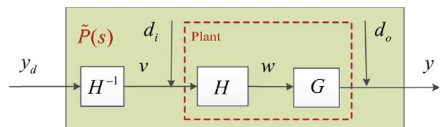
Fig. 1. The block diagram of hysteresis compensation.
