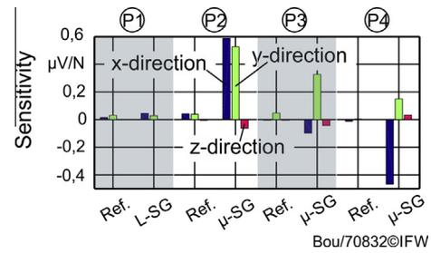
Fig. 3. Influence of the notches on the sensitivity to load.
