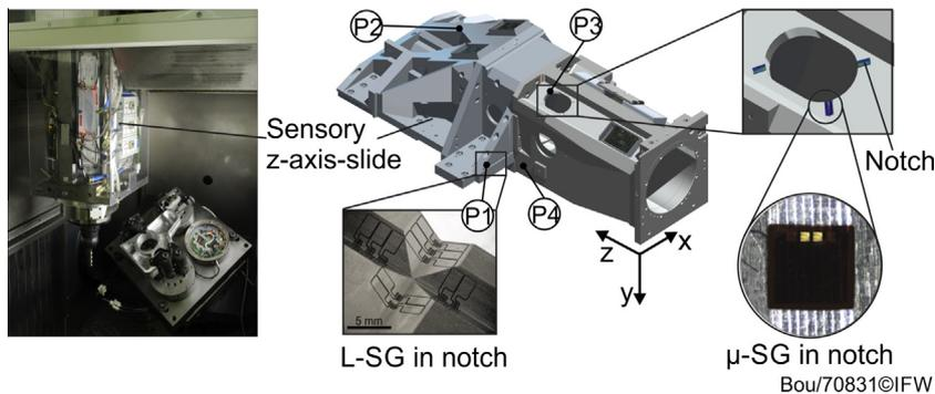
Fig. 2. Integrated sensory z-slide in the test machine tool.
