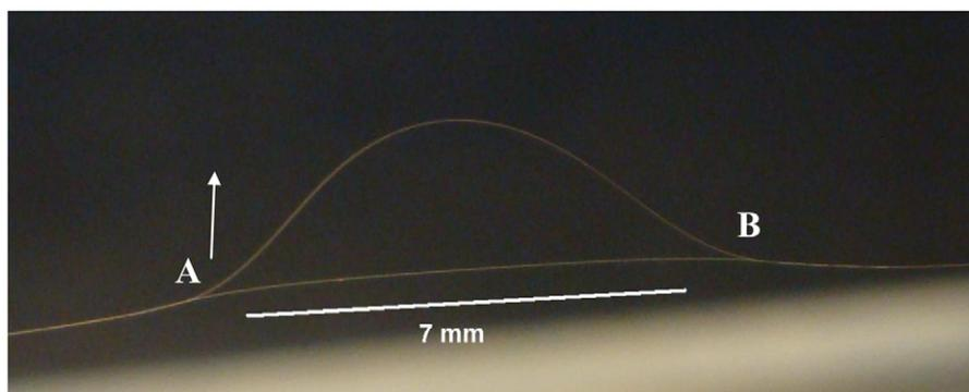
Fig. 3. Unpackaged MMZI structure fabricated using a flame brushing technique.
