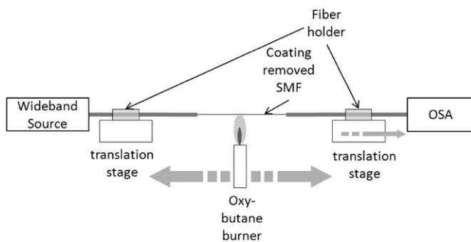
Fig. 1. Microfiber fabrication setup.
