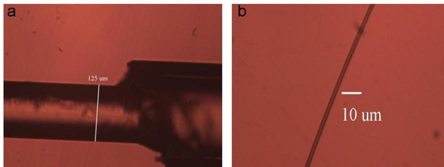
Fig. 2. Optical microscope image of (a) the stripped un-tapered fiber and the fabricated microfiber.
