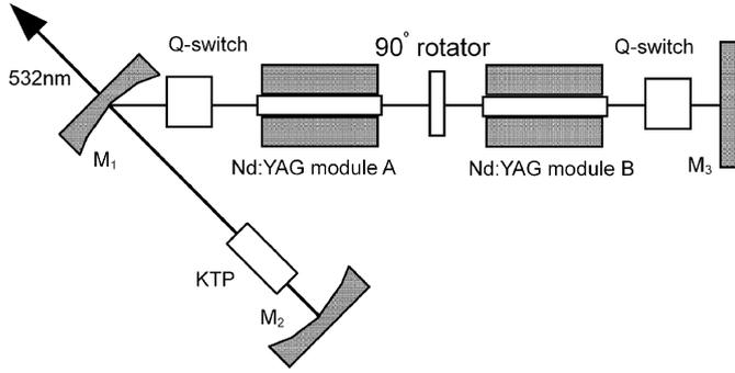
Fig. 1. Schematic drawing of the cavity configuration.
