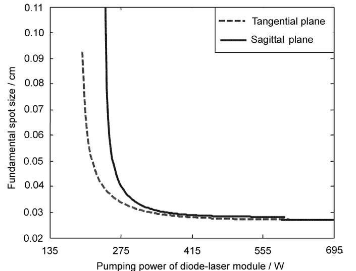
Fig. 2. Variation of fundamental spot size on folded mirror with pumping power.
