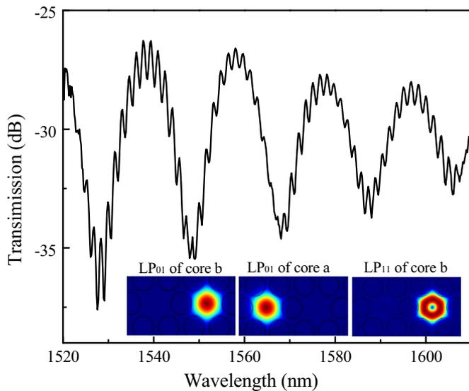
**Fig. 2.** Transmission spectrum of the sensor (insets: mode profile of the LP01 mode of core A and core B, and of the LP11 mode of core B).
