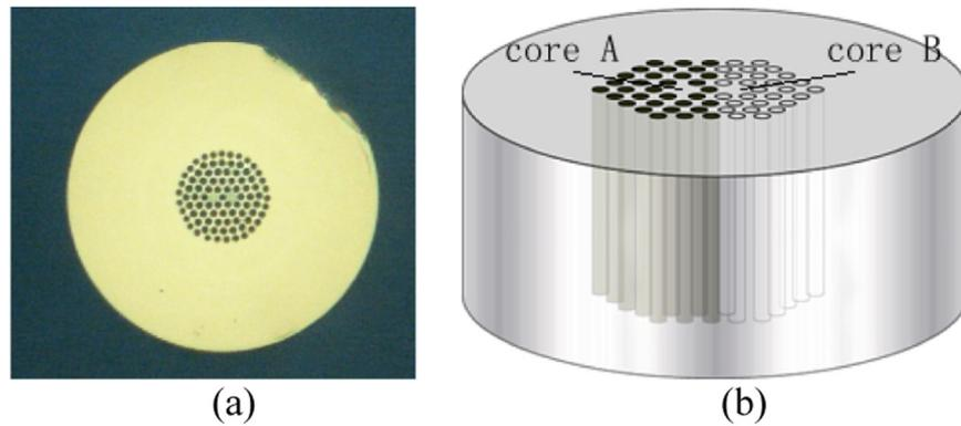
**Fig. 1.** (a): The cross section view of the twin core PCF. (b): Schematic illustration of the asymmetrically infiltrated twin core PCF.
