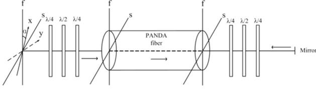
Fig. 2. Illustration of the polarization state of the propagation light in the quasi-Sagnac interferometer.
