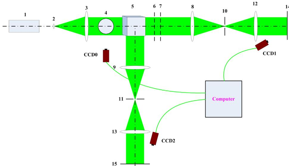
1-Laser (532nm), 2-Extender lens, 3-Collimating lens, 4-flow field,
