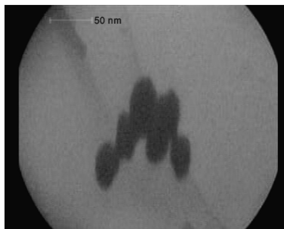
Fig. 1. TEM image of gold nanoparticles.
