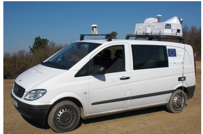
Fig. 2. The Lynx Mobile Mapper system used to collect the test datasets.
