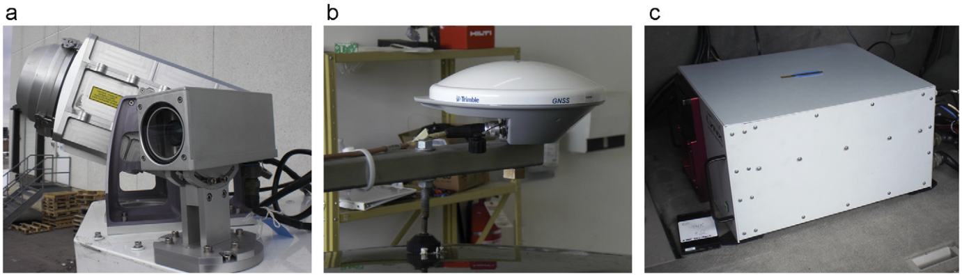
Fig. 1. (a) Lynx LiDAR sensor and camera. (b) Applanix GPS antenna deployed on the vehicle and (c) Lynx control unit.
