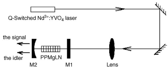
Fig. 2. The experimental setup of an OPO system. The pump laser was an AO Q-switched Nd:YVO<sub>4</sub> laser working at 1064 nm. M1 is the input mirror and M2 the output mirror. The substrate of both mirrors is CaF<sub>2</sub> crystal.
