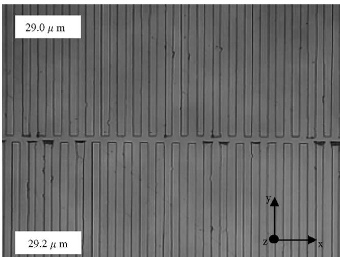
Fig. 1. The optical microscopic image of etched PPMgLN surface. It shows the +Z surface of PPMgLN after it has been etched in a 40% hydrofluoric acid at room temperature for about 1 h.
