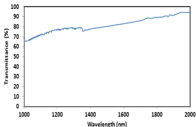
Fig. 3. Transmission curves of MWCNTs-PEO film.
