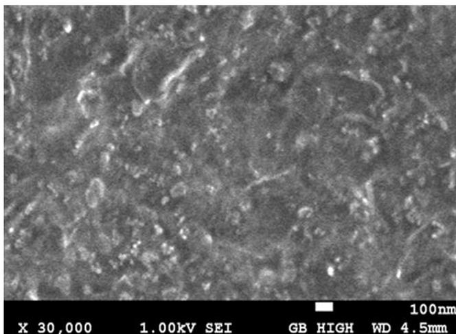
Fig. 1. FESEM image of the MWCNTs-PEO thin film absorber (30,000 $\times$  magnifications).
