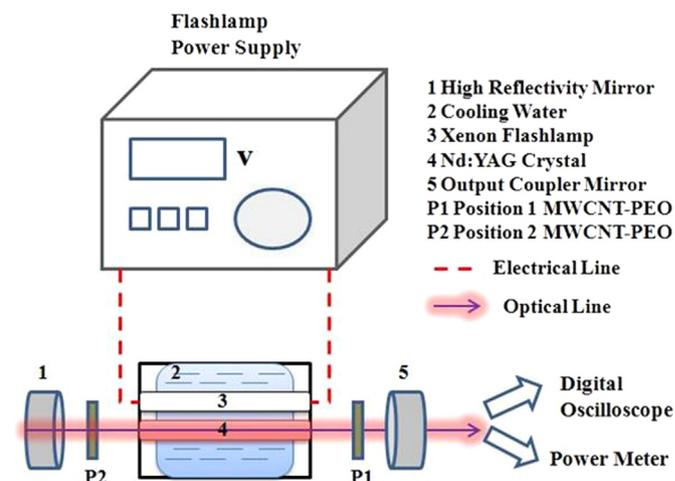
Fig. 4. Schematic diagram of the experimental set-up.
