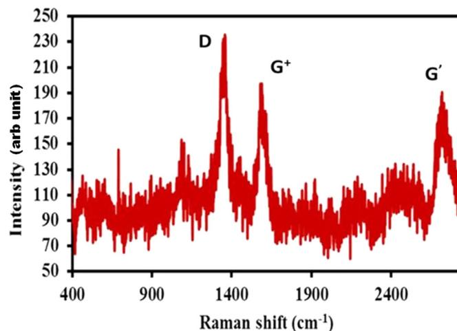
Fig. 2. Raman spectroscopy of MWCNTs-PEO film.
