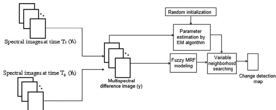
Fig. 1. Diagram of the proposed change detection scheme.
