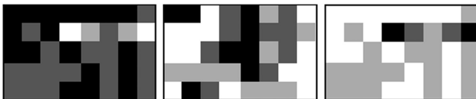
Fig. 1. Hypotheticals THSP with (a) high occurrence of dark pixels, with (b) the grey levels randomly distributed, and with (c) high occurrence of light pixels.
