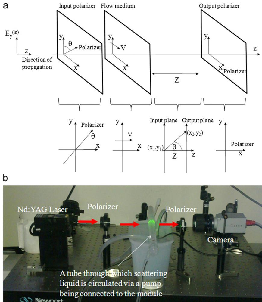
Fig. 1. Schematic sketch of experimental setup (a) and image of experimental setup (b) including laser, first polarizer, flow system, second polarizer (analyzer) and camera.
