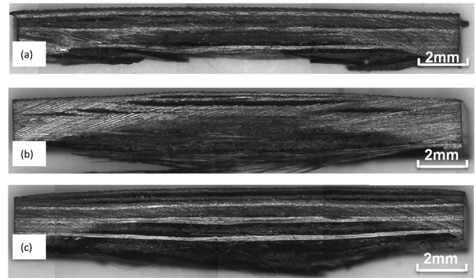
Fig. 2. Cross section for the cases of laser power (a) 500 W, (b) 800 W and (c) 1000 W.
