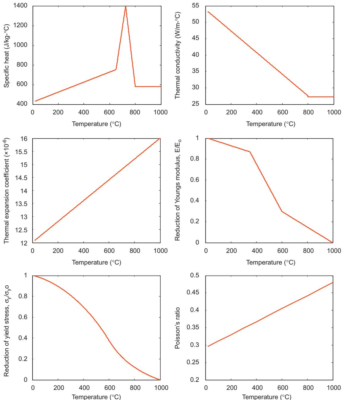
Fig. 1. Thermal and mechanical properties of low carbon steel.
