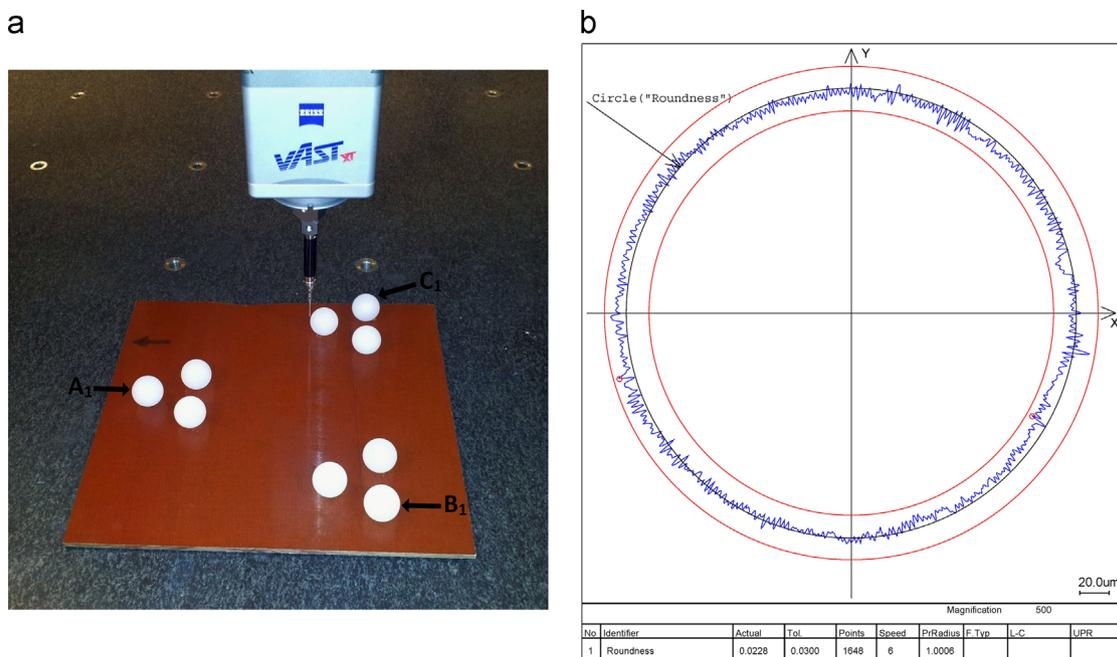
Fig. 1. Spheres calibration board: (a) calibration board on CMM and (b) representative roundness of calibration balls.
