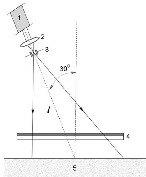
Fig. 2. Optical arrangement for recording reflection hologram for one of the channels, where: (1) is the He–Ne laser, (2) beam expander (micro objective), (3) spatial filter, (4) holographic plate, (5) diffuse light reflective metal screen.
