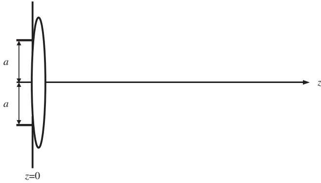
Fig. 1. Schematic illustration of pulsed Bessel beams focused by an aperture lens.
