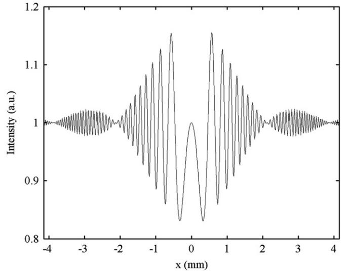
Fig. 1. Simulated in-line hologram of the spherical particle with the size  $2a = 124.96 \mu\text{m}$  and the axial distance  $z = 40 \text{ cm}$ .
