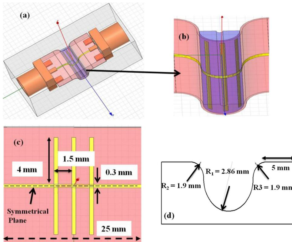
**Fig. 1.** (a) HFSS layout of the proposed microwave/microfluidic sensor filled with liquid solution. (b) Zoom image of the bended section of (a). (c) HFSS layout of straight structure to present the dimensions of the sensor. (d) Dimensions of the 3D-printed ABS plastic support.
