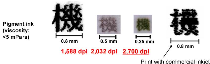
**Fig. 3.** Print samples of Chinese character “mecha” by using the electrostatic inkjet and a commercial inkjet (material: pigment ink).
