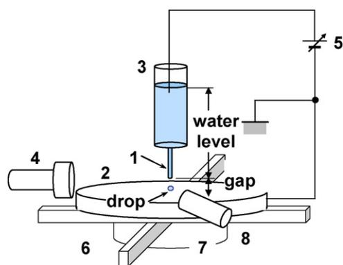
**Fig. 1.** Experimental set-up of electrostatic inkjet (1. water pin electrode, insulative capillary tube filled with ink; 2. metal plate electrode; 3. ink tank; 4. high-speed camera; 5. high voltage amplifier and function generator; 6. linear stages, x and y directions; 7. mechanical z-stage; 8. light).
