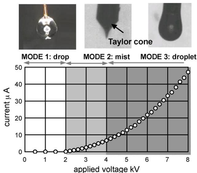
**Fig. 2.** *V*–*I* curve in pin-to-plate electrode system and modes of drop formation (3 mm air gap).
