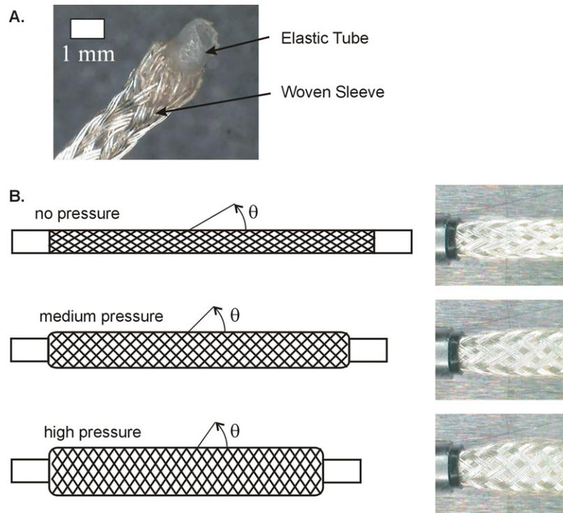
Fig. 1. (a) Example of a McKibben actuator developed during this research. (b) Operation principle of McKibben actuators.
