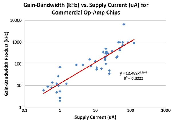
Fig. 2. Gain-bandwidth vs. supply current for a number of commercially-available amplifier ICs, from Sherman [25].
