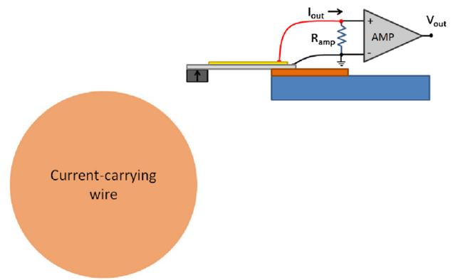
Fig. 1. Side view of a piezoelectric permanent magnet current sensor, close to a current-carrying wire, from Sherman [25].
