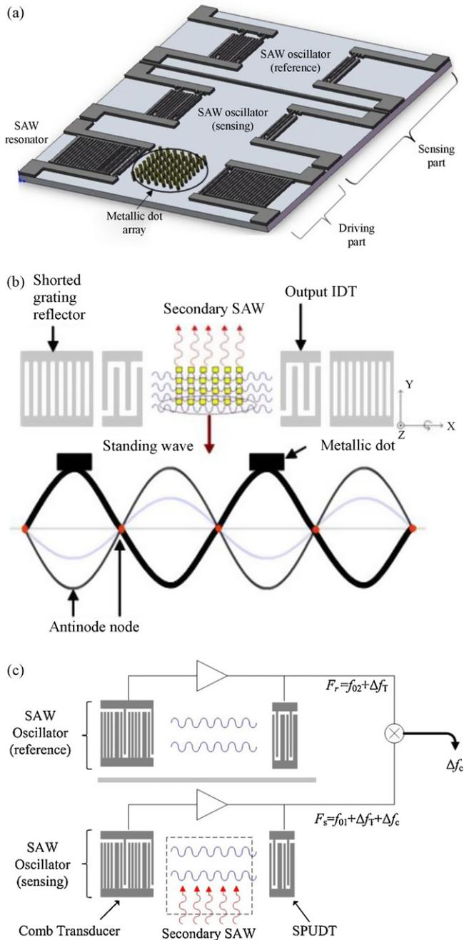
**Fig. 1.** (a) Entire view of the SAW gyroscope. (b) Magnified views of the driving part and (c) sensing part.
