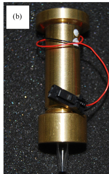
Fig. 2. The novel printhead: (a) schematic showing of the design (out of proportion). (b) A self-fabricated printhead following the novel design.
