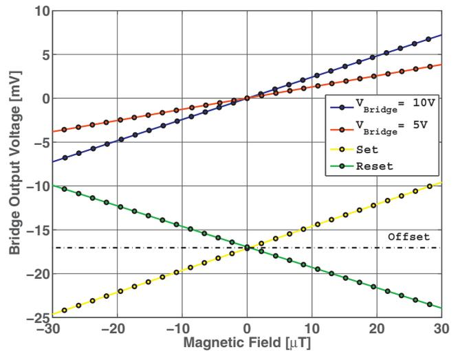
**Fig. 1.** Output characteristics as a function of the magnetic field after a *set* (yellow trace) and *reset* (green trace) pulse with  $V_{\text{bridge}} = 10 \text{ V}$ . Bridge offset extraction is performed for  $V_{\text{bridge}} = 10 \text{ V}$  (blue trace) and  $V_{\text{bridge}} = 5 \text{ V}$  (red trace). (For interpretation of the references to color in this figure legend, the reader is referred to the web version of this article.)
