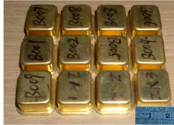
Fig. 2. The metallic packages for vacuum packaging experiments.
