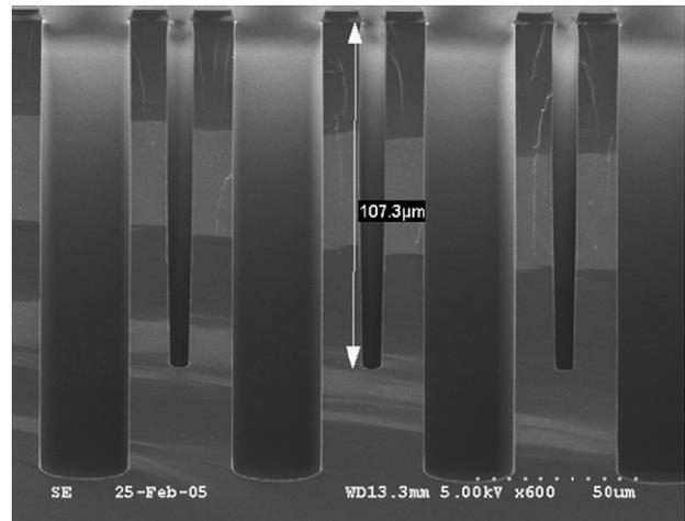
Fig. 2. SEM of trenches with two different widths demonstrating the effect of aspect ratio on the trench profile. Trenches with higher aspect ratio start to pinch-off at the bottom as a result of insufficient passivation layer removal.
