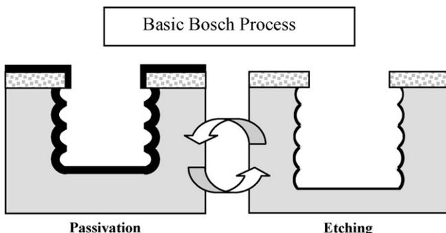
Fig. 1. Schematic viewgraph of the basic Bosch process.
