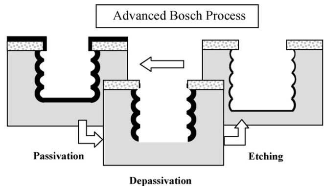
Fig. 3. Schematic viewgraph of an advanced three-pulse Bosch process.
