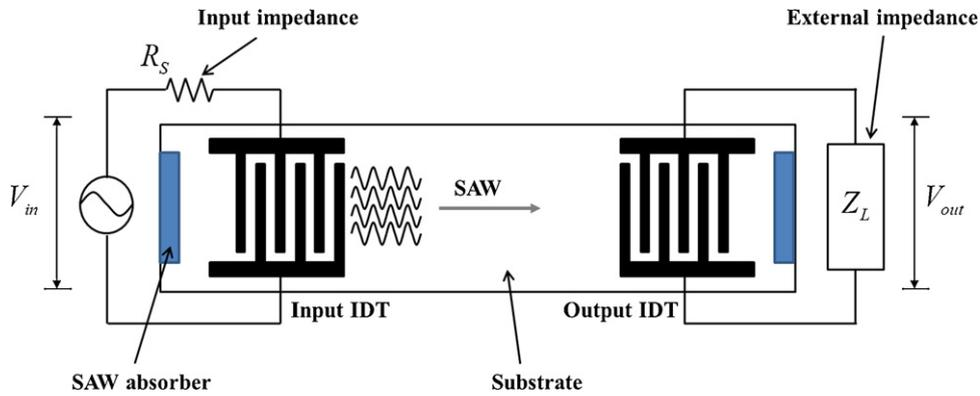
Fig. 1. Structure of the SAW device used as a signal conditioner with an external impedance  $Z_L$ .
