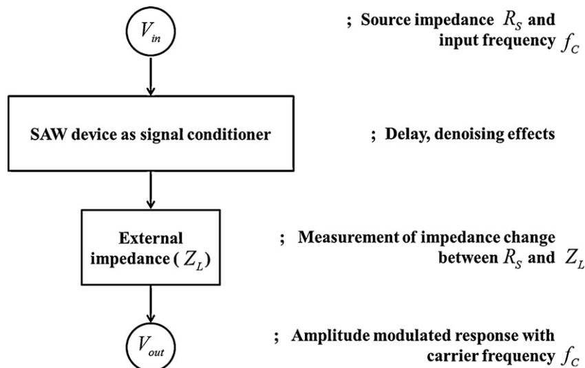
Fig. 2. Overall signal flow of measurement system.
