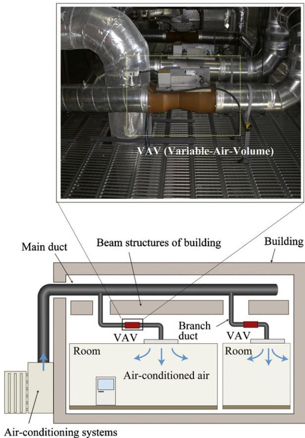
Fig. 1. Variable-air-volume unit and large-scale building air-conditioning system.
