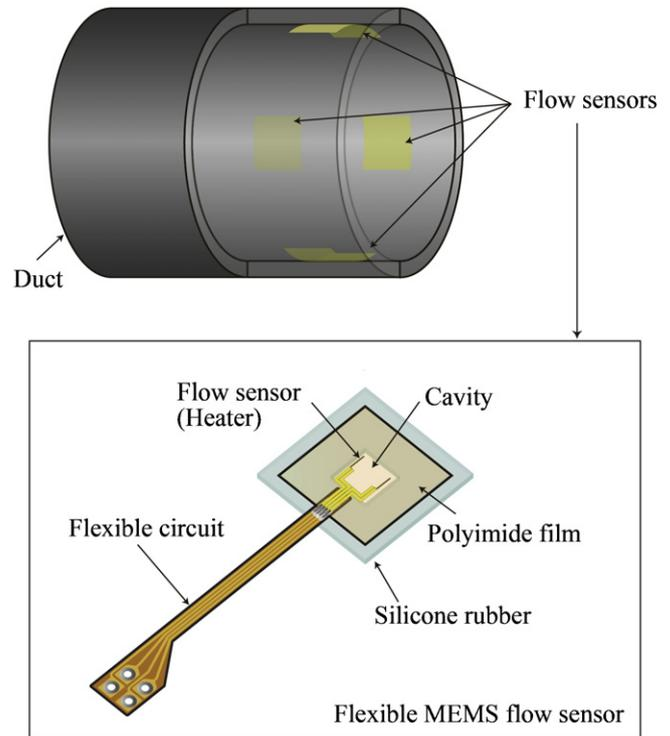
Fig. 2. Flexible MEMS flow sensor and its position on inside surface of duct.
