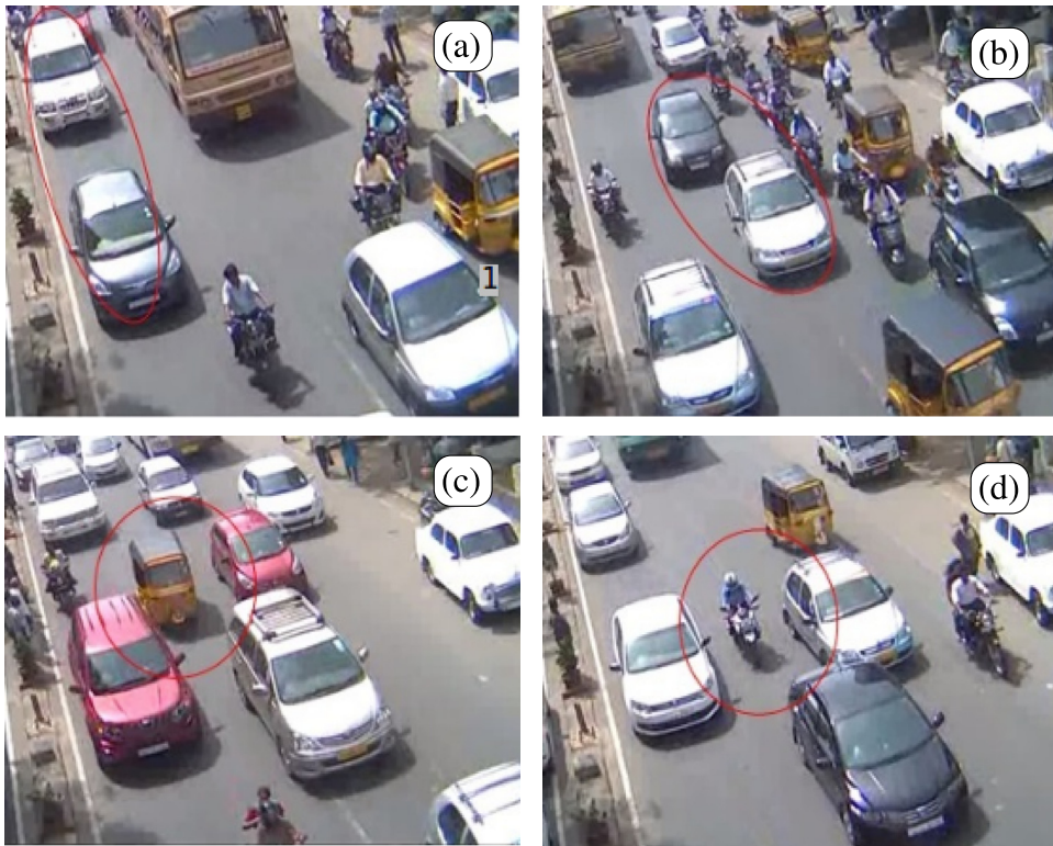
Fig. 1. The four driving behavioral patterns of mixed traffic. (a) In-line car following, (b) staggered following, (c) following between two vehicles, and (d) passing.
