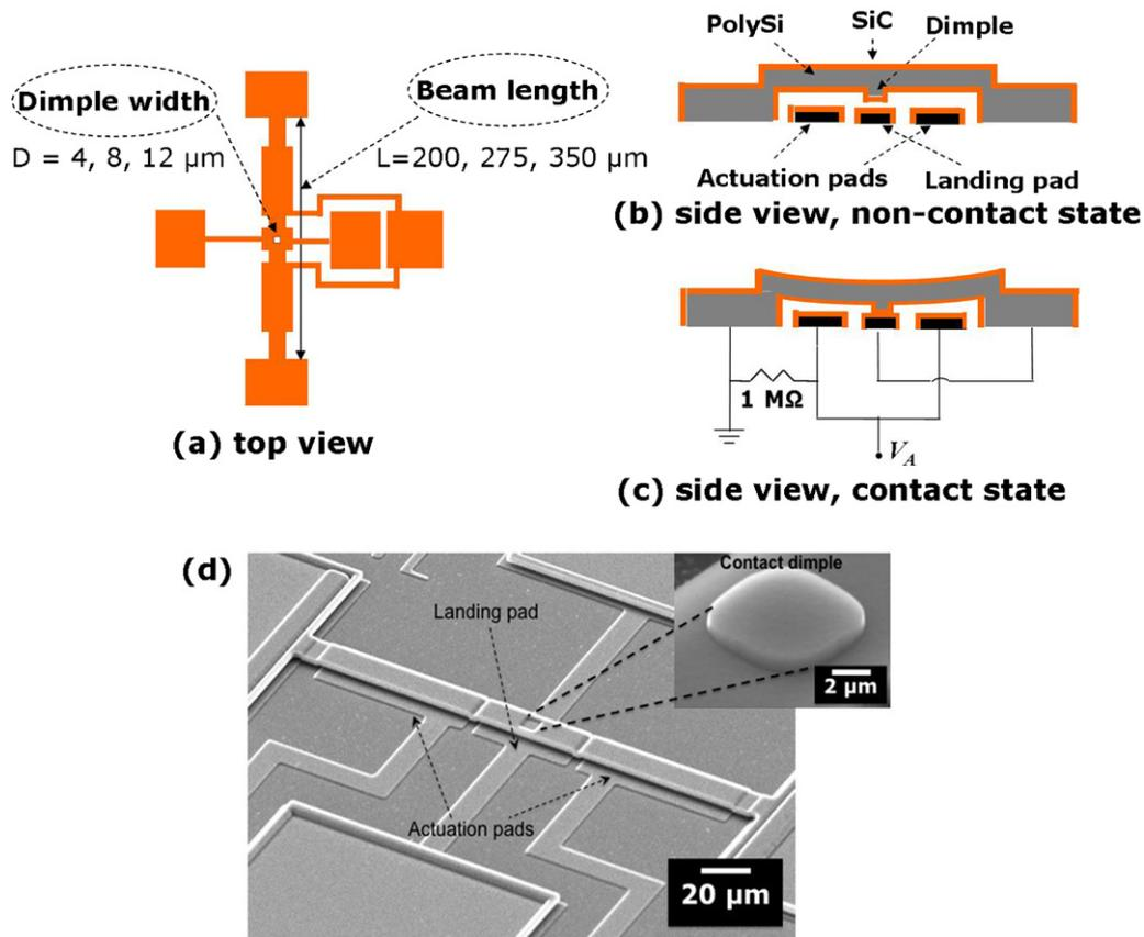
**Fig. 1.** (a)–(c) Schematic representations of the electrostatically actuated double-clamped beam test structure. The same designs were also coated with a polycrystalline SiC film for comparison. (d) Representative SEM micrograph of a  $275\ \mu\text{m}$  long polysilicon DCB device (inset is an inverted dimple).
