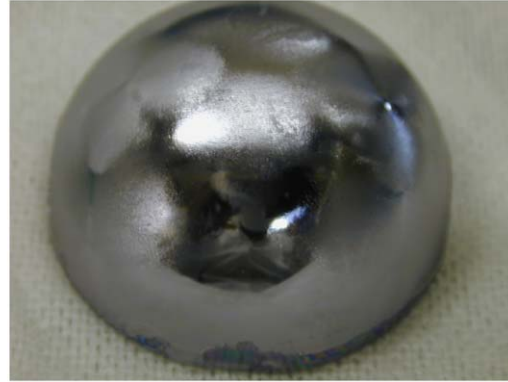
Fig. 1. Hemispherical single-crystal silicon specimen to evaluate for a number of crystallographic orientations: (a) schematic diagram and (b) photograph of the specimen after etching.
