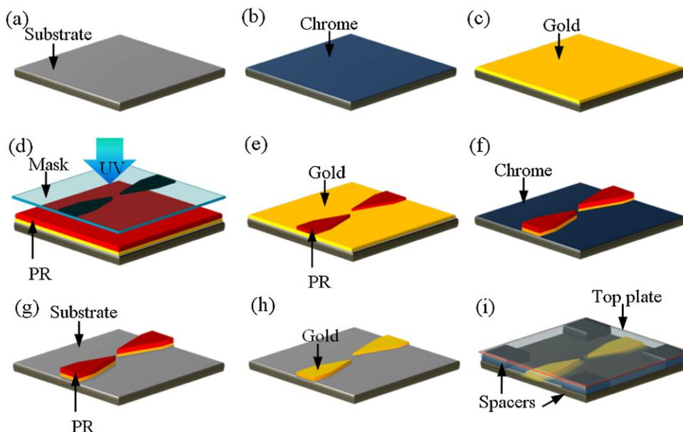
**Fig. 2.** Microfabrication steps of chips used for testing.
