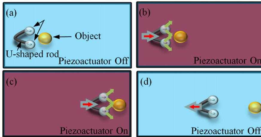
**Fig. 1.** Micro-object manipulation by acoustically excited identical twin bubbles: (a) initial state; (b) when identical bubbles on the tips of a U-shaped rod are acoustically excited, they simultaneously oscillate and generate microstreaming, which, in turn, pushes an object; (c) the rod moves to the right, and the object is carried by the microstreaming; (d) the excitation is turned off and the rod moves to the left; the object is released from the bubbles and remains at its position.
