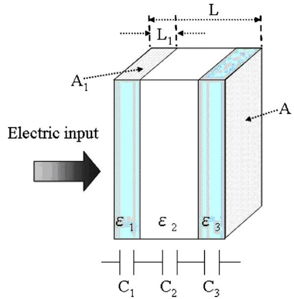
Fig. 2. Diagram of the three-layer model.
