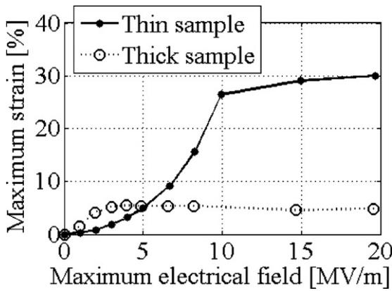
Fig. 1. Two typical variations of strain versus applied electrical field for a polyurethane film; thin (28  $\mu\text{m}$ ) and thick (140  $\mu\text{m}$ ) samples.
