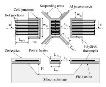
Fig. 1. Schematic top view (upper) and cross-section (lower) of the simulated flow meter (not to scale).
