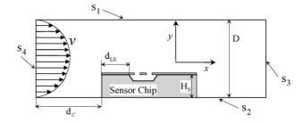
Fig. 2. Two-dimensional configuration used to represent the experimental case.
