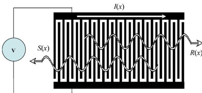
Fig. 2. SAW schematic and variables for COM theory of the IDTs.
