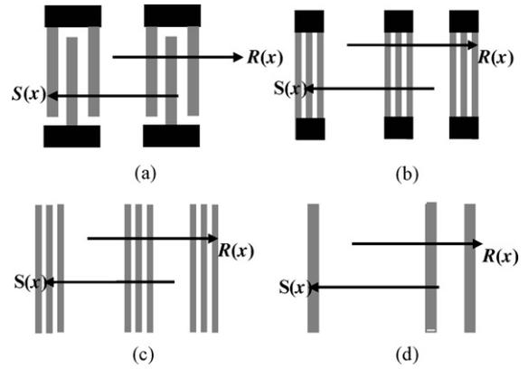
Fig. 3. Reflectors for the SAW reflective delay line: (a) IDT type, (b) shorted circuit grating reflector, (c) open circuit grating reflector and (d) bar type reflector.
