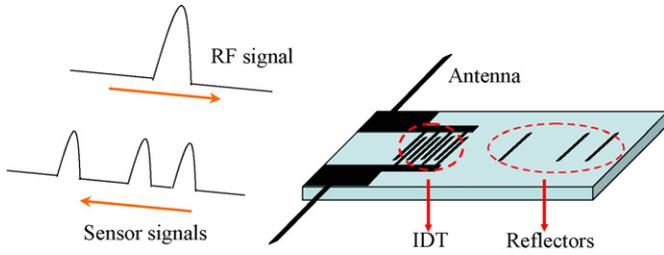
Fig. 1. Schematic diagram of the SAW-based pressure sensor.
