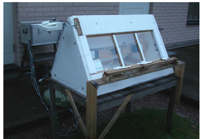
Fig. 2. Picture of Sample Test Box. Three glass samples are mounted on the front. The lasers, each one pointing at a glass surface, are on the board in front of the box. The three detectors are inside the box.
