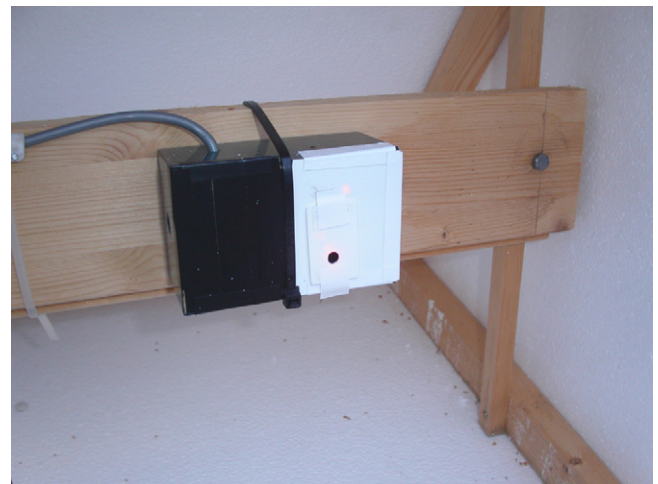
Fig. 3. Close-up of one of the detectors. The detector is shielded with a box so that as little stray light as possible reaches the detector.
