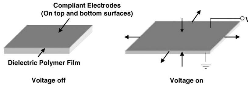
Fig. 1. Principle of operation of a dielectric elastomer actuator.
