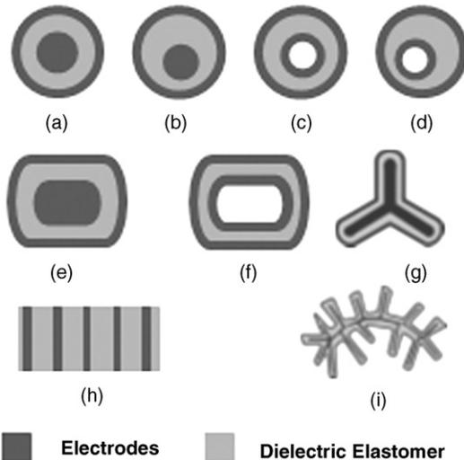
Fig. 2. Cross-sectional shapes of various multicomponent fibers as potential actuators. (a) Concentric: sheath/core; (b) eccentric: sheath/core; (c) hollow concentric: sheath/core; (d) hollow eccentric: sheath/core; (e) ribbon; (f) ribbon-hollow; (g) trilobal; (h) segmented ribbon; (i) multicellular-irregular.
