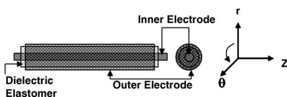
Fig. 3. Schematic of the fiber actuator showing placement of dielectric material and compliant electrodes.
