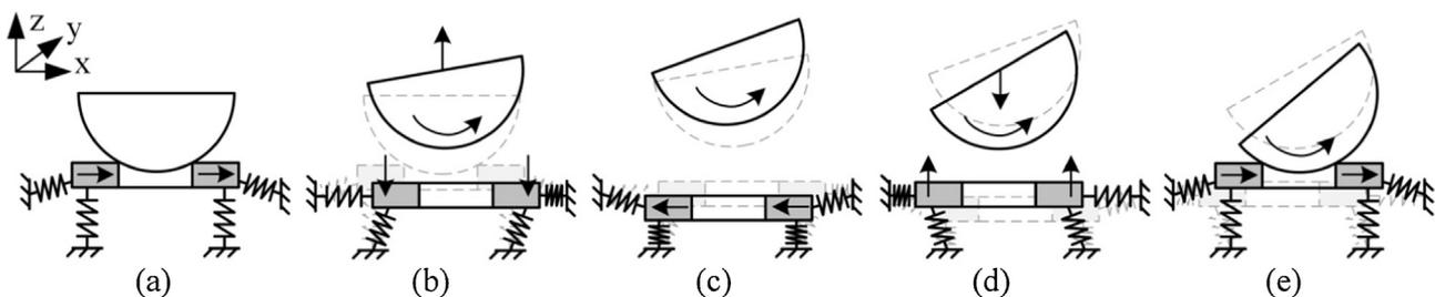
**Fig. 2.** Stage-hemisphere interaction for a rotation around the  $y$ -axis. The stage oscillates elliptically clockwise and hits the hemisphere at its highest position. The momentum transfer results in a  $z$ -movement and an anticlockwise rotation of the hemisphere.
