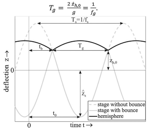
**Fig. 3.** Desired movement of the stage (grey solid line) and the hemisphere (black solid line) for  $f_s/f_g = 3/5$  in comparison to the stage oscillation without bounces (grey dashed line).
