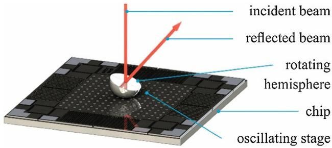
**Fig. 1.** Schematic setup for quasi-static laser beam deflection. The incident beam is reflected on the plane surface of a hemisphere, which is rotated due to the stage movement.
